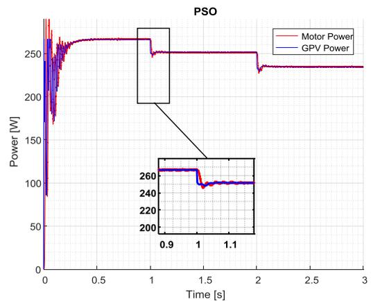
Fig 14. Variation of the PVG power and Motor power (W)
