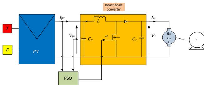
Fig 2. DC-DC Boost converter
