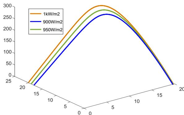
Fig 4. P-V-I output characteristics of PV array.
