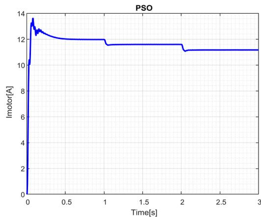
Fig 16. Variation of the motopump current.
